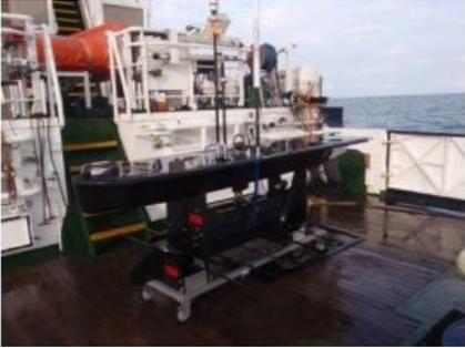
In what is believed to be a world's first in the scientific community, Cefas (Centre for Environment, Fisheries and Aquaculture Science, UK) and Liquid Robotics, USA, have successfully deployed, tested and recovered a remotely piloted [Wave Glider](#). This allowed scientists to measure water characteristics and selectively collect samples in near real time.
