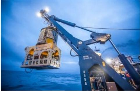
Reliable navigation and positioning underpin productive use of submerged vehicles, leading to optimized operations, expanded capabilities, and greater cost-effectiveness. For 25 years, Teledyne RDI Doppler Velocity Logs (DVLs) have been an industry-leading solution for this need. DVLs are sonar systems that accurately measure a vehicle's speed over ground and altitude above the seabed.
