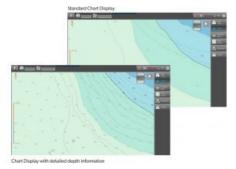
ORCA Pilot Chart Mapper is a new complementary tool for SevenC's PPU software, ORCA Pilot G2. It has been developed to make pilots more independent, flexible and up to date when it comes to high-precision charts in local areas. Chart Mapper creates an optional chart layer with high-density depth information for display in a PPU within seconds!
