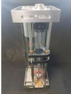
UK-based Ocean Scientific International (OSIL) has announced the release of an innovative new sediment corer designed to be mounted to the skids of ROVs or AUVs. The self-contained system will allow sediment samples to be collected during routine ROV operations and can be daisy chained together to allow multiple core assemblies to be installed as one system.
