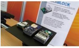
Iridium satcom specialist Rock Seven is introducing a compact plug & play two-way satellite communications system with integrated antenna at Ocean Business 2017 in Southampton (at stand V43). Utilising the latest Iridium modem technology, Rock Seven engineers have managed to shrink the compact RockBLOCK form factor down to just 45mm x 45mm x 15mm, including its antenna.
