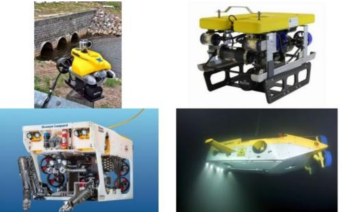
The concept of ROVs does not seem to change too much over time. Basically, they are self-propelled instruments working in deep waters up to about 6,000m that are linked to a vessel-based controller. This distinguishes them from AUVs that move underwater without a tether to a vessel. As with any other machine, they are available in many shapes and types, evolving over time. With a hydrographer's eye, we give an overview of the varieties available and the direction in which ROVS are moving.
