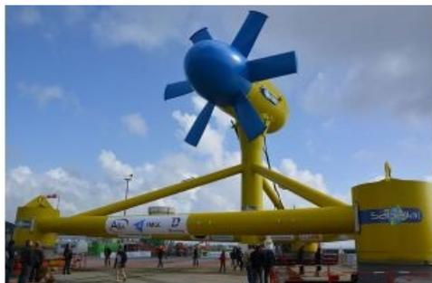
The environment of the Sabella D10 tidal turbine, including underwater sounds, currents, wave, etc., is analysed using a sensor system developed by RTsys (France). Having been tested over the course of a year, between 2015 and 2016, Sabella D10 will be submerged once again in spring 2017 for further testing in the Fromveur Passage, off the coast of Brittany.
