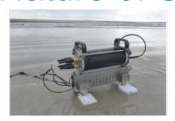
How can you study sea-floor sediments simply, quickly and without taking samples? RTsys answers this question with acoustics. The French company, a specialist in underwater electronics and acoustics, has perfected INSEA (INvestigation of SEdiments by Acoustics), a sound velocity meter intended for studying sediments.
