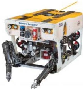
Saab Seaeye has further enhanced its system for global remote control of its electric underwater robotic vehicles via satellite link and 4G networks. Remote control of the [Leopard](#) electric robotic work vehicle has now been upgraded to include control of the TMS. Such remote operations will bring considerable savings to the oil and gas industry by reducing the need for offshore piloting personnel and
