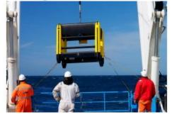
MacArtney has supplied a second <u>Triaxus</u> ROTV for use on the research vessel *RV Investigator*. This Triaxus E version features an even higher payload capacity and enables the installation of a wide range of sensors targeted to the specific needs of oceanographic research.
