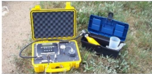
Aquatec Group has expanded the 'Sediment? Solved' range to include instrumentation to measure surface sediment stability, with the addition of Partrac's benthic flumes and Cohesive Strength Meter (CSM). The Cohesive Strength Meter is a field instrument that directly measures the surface erodibility of marine, fluvial and terrestrial sediments. It
