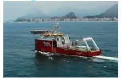
Brazil's most advanced ROV support vessel (RSV), the '*Fugro Aquarius*', is using specified acoustic positioning technology supplied by Sonardyne Brasil Ltda. to support its subsea inspection, repair and maintenance activities in the region. Already delivered and fully commissioned, the Ranger 2 Ultra-Short BaseLine (USBL) system is being used to track the precise position of the vessel's work-class ROVs in water depths of up to 3,000 metres.
