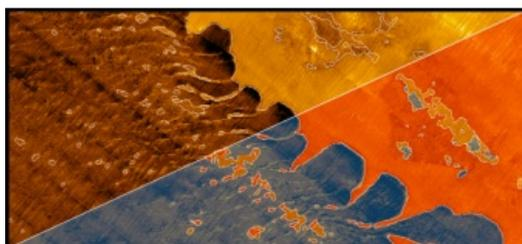
One feature of SonarWiz 7 is the Seabed Characterisation tool. It incorporates bathymetric slope, roughness, TPI and any spatially distributed variable that can aid the characterisation algorithm to generate classes of texture.
