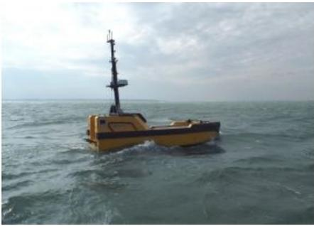
ASV Global has announced the successful deployment of one of its C-Worker 7 class of autonomous surface vessels for Subsea 7. The 7m autonomous surface vessel was used to support a pipelay operation off the coast of Egypt. Fitted with a survey suite comprising a multibeam echosounder and sidescan sonar, the C-Worker 7 carried out touchdown monitoring in support of the 'Seven Antares' pipelay vessel.
