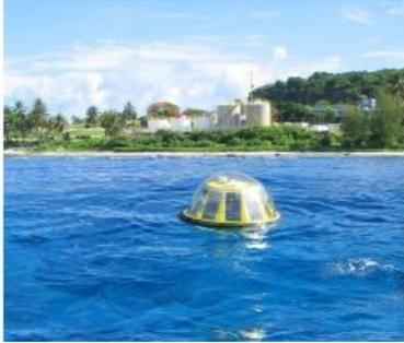
AXYS Technologies' TRIAXYS g3 wave sensor has successfully completed a series of rigorous sea trials. The trials were conducted both in the German Bight and off the West Coast of Canada and used both AXYS' own TRIAXYS wave buoy and other industry standard buoys as references. The TRIAXYS g3 [demonstrated high levels of correlation](#) against all reference buoys, confirming that the TRIAXYS g3 sensor meets AXYS' high standards of accuracy for wave height and direction measurement.
