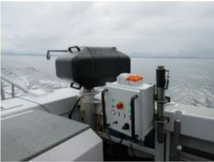
US-based Teledyne Oceanscience has announced the launch of rapidCAST, an automated sound velocity (SV) profiling system for moving vessels. With the capability to automatically cast and recover a high-quality SV probe to 500 metres at 8 knots without an operator on deck, rapidCAST offers many of the benefits previously only available from large towed profilers. Simultaneously, it offers surveyors the convenience and cost savings of a small and portable unit that is easy to mobilise.
