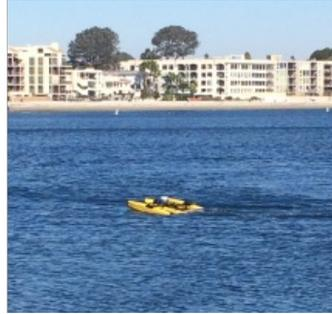
The Teledyne Oceanscience Z-Boat 1250 is a remotely operated hydrographic survey boat that is sturdy enough for tough terrain but light enough to be one-person portable. It is outfitted with a singlebeam echosounder and is suited for inland waters such as streams, rivers and lakes.
