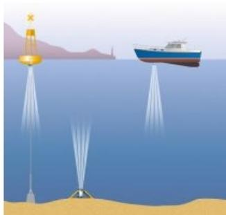
Acoustic Doppler Current Profilers (ADCPs) are sonar systems that measure water current velocities. The Doppler effect allows the sensors to measure the velocities over a range of depths, making them ideal for measuring currents in oceanographic applications. [Geo-matching.com](http://Geo-matching.com), the product comparison platform where hydrographic and geospatial professionals can find and
