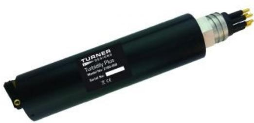
Turbidity measurements are often made in shallow waters and keeping the instrument optical face clear is particularly important. Turner Designs has introduced a turbidity sensor addressing this issue with a simple solution. Turbidity Plus is an accurate single-channel turbidity sensor including an integrated wiper which is triggered by the user.
