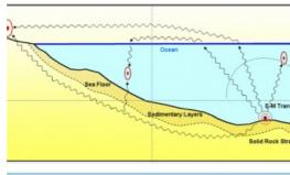
Underwater wireless communications links have almost exclusively been implemented using acoustic systems. Optical links have proved impractical for many applications. Although underwater radio links were experimentally evaluated in the pioneering days of radio, they did not meet the requirements of the time. Given modern operational requirements and digital communications technology, the time is now ripe for re-evaluating the role of electromagnetic signals in the underwater environment.
