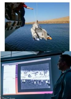
This article presents the development, production and testing of wireless underwater acoustic video communications, which is unique in the world today. It also discusses the implementation of this technique on Autonomous Underwater Vehicles (AUV's) to perform inspections of underwater oil and gas pipelines. The achieved characteristics, limitations and upcoming prospects are presented.
