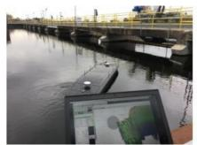
Inspection of dams is a high-risk task for divers because of strong currents and eddies. The use of emerging technologies such as uncrewed surface vehicles equipped with echosounders and sonars can lower those risks. Such systems can perform subsurface dam inspections quickly and effectively without putting humans at risk, as this US case study shows.
