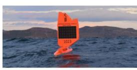
A 7m (23ft) long, wind-powered <u>unmanned surface vehicle (USV)</u> has become the first unmanned system to circumnavigate Antarctica. Known as SD 1020 and equipped with a suite of science-grade sensors, the vehicle collected data in previously uncharted waters, enabling new key insights into ocean and climate processes.
