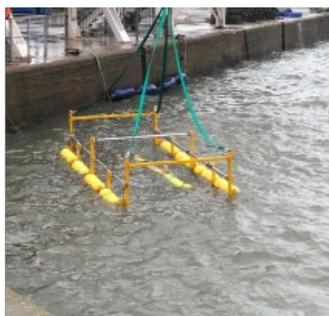
UTEC, a global surveying company in subsea services group Acteon, has commissioned its launch and recovery system (LARS) for the fleet of seven autonomous underwater vehicles (AUV) it uses for seabed surveys in the oil and renewables industries.
