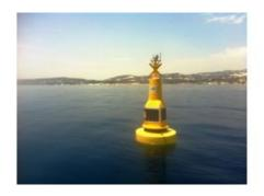
UK-based Ocean Scientific International Ltd (OSIL) have recently supplied a 1.2m Tern Buoy to Gardline Environmental, for installation in Cyprus. The buoy is equipped with a Nortek AWAC, acquiring full profile current speed and direction and wave data in addition to other ancillary parameters including GPS positioning. Data from the AWAC is currently transmitted via GSM. However, the buoy has also been equipped with the option to swap comms to Iridium satellite.
