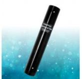
The AQUAscat 1000LT acoustic profiler by Aquatec (UK) has been developed to make measurement of suspended sediment easier. The AQUAscat 1000LT observes profiles of suspended sediment concentration of up to 2.5m using multi-frequency acoustics. Profiling allows sediment dynamics such as re-suspension and entrainment to be explored, which is not possible with single point measurements.
