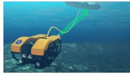
Subsonus Tag is a new acoustic positioning transponder that operates with the Subsonus USBL. It was developed to provide a low-cost, fully integrated positioning capability to users across a broad array of applications. It features an integrated battery and a revolutionary acoustic processing architecture that allows it to operate for up to 18 months on one charge.
