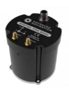
Advanced Navigation releases their GNSS/INS Spatial FOG Dual, a new variant of the Spatial FOG product featuring the addition of high-accuracy dual antenna heading. The system operates with two GNSS antennas that are mounted fore and aft on the vehicle. By continuously measuring the phase difference of the GNSS signal received on each of the antennas, it is able to calculate the bearing between the two antennas which provides a very high accuracy heading source.
