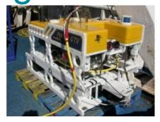
Ageotec, Italy, has delivered to Cadden (France) its first Perseo GTV. The Perseo GTV fills a gap in deep-sea survey and intervention ROV operations, being an alternative to existing higher-class vehicles whenever cost-effective solutions are required in terms of shipping, handling and vessel support. It can include payloads like multi-beam echosounders and cutters or manipulators.
