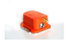
The MTi-G is a MEMS IMU with integrated GPS. It contains an internal ultra low-power Attitude and Heading Reference System (AHRS) processor running a real-time Xsens Kalman filter. Key benefit of the compact MTi-G sensor is that it provides accurate horizontal and vertical position, velocity and orientation estimates.
