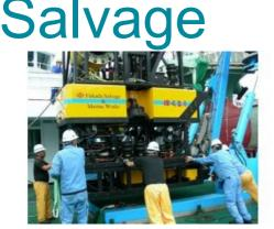
International Submarine Engineering, Canada, is pleased to announce the contract to build a 50HP 3,000mdepth Hysub ROV for Fukada Salvage and Marine Works, Japan. The Fukada Hykuyo Hysub 50-3000 is a versatile and capable medium duty work-class ROV. The vehicle will be outfitted with two manipulators, one 7-function and one 4-function along with assorted tooling for a broad range of operational capabilities.
