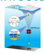
ASL Environmental Sciences has announced the combining of its <u>Acoustic Zooplankton Fish Profiler</u> (AZFP) with its Ice Profiling Sonar (IPS) to provide a comprehensive solution for ice thickness detection and water column profiling of fish, zooplankton, bubbles and suspended sediments in ice-infested waters.
