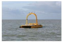
Current plans for ASV's partly solar-powered vehicle C-Enduro include coastal operations off Scotland's east coast as well as inland loch surveys. The C-Enduro will also be used as a platform for interacting with other unmanned systems such as autonomous underwater vehicles (AUVs). This was announced during Ocean Business, which is continuing today in Southampton, UK.
