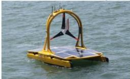
Heriot-Watt Universityâ€<sup>™</sup>s Edinburgh Campus (UK) has confirmed the order of an ASV C-Enduro. The C-Enduro Unmanned Surface Vehicle (USV) will be used for research in persistent and long-term autonomy with multiple remote and autonomous marine platforms. The vehicleâ€<sup>™</sup>s primary application will be as a moving navigation and communication platform for AUVs.
