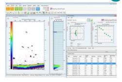
BioSonics, USA, has released VisAcq AutoTrack, a software module for researchers who use hydroacoustics for stock assessment of fisheries. VisAcq AutoTrack calculates the sampled volume and fish density by depth strata. At the conclusion of a mobile hydroacoustic survey, data processing is essentially completed and the user need only export track lists to a CSV file.
