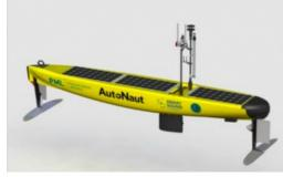
An AutoNaut uncrewed surface vehicle (USV) equipped with a range of scientific sensors has been acquired by Plymouth Marine Laboratory. The state-of-the-art 5m craft is powered entirely by renewable energy and will be the first USV to regularly run scientific missions off the coast of the UK.
