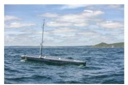
A pioneering project to find out how increasing levels of man-made noise in the sea is affecting marine life has begun in Plymouth. Plymouth University Marine Institute scientists are working with AutoNaut and its 5m wave-propelled <u>unmanned surface vessel (USV)</u>, towing a Seiche passive acoustic monitoring (PAM) array.
