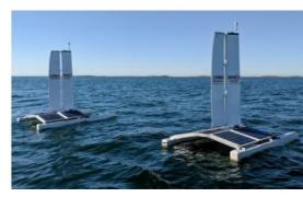
Norwegian offshore wind developer Equinor and US-based start-up Autonomous Marine Systems (AMS) have launched a 16 ft autonomous sailing platform to cut the cost of gathering data needed for developing offshore wind projects. The wind and solar-powered Datamaran vessel, developed by AMS, carries a LiDAR device to collect data on wind and weather conditions at remote offshore wind lease areas.
