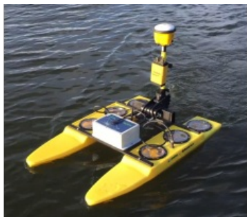
survey catamaran platform for bathymetric surveying.
