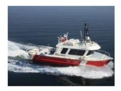
ASV Global has converted a 26ft hydrographic survey launch to enable it to operate autonomously using the ASView control system, while maintaining its ability to operate in a conventional manned mode. The launch, which is part of the Canadian Coast Guard's (CCG) fleet dedicated to the survey operations of the Canadian Hydrographic Service (CHS), will be used as a test platform for unmanned survey work.
