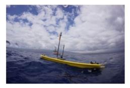
In partnership with Boeing, the world's largest aerospace company, the Australian Institute of Marine Science (AIMS) has demonstrated how an autonomous ocean vehicle, the Wave Glider, can improve monitoring of the Great Barrier Reef and coastal waters.
