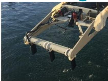
Innovatum have successfully tested Smartrak, a fully autonomous passive magnetic tracking system of a submarine cable by Autonomous Underwater Vehicles (AUV). An AUV Data Protocol has also been developed providing a standard communication format between Smartrak and the AUV.
