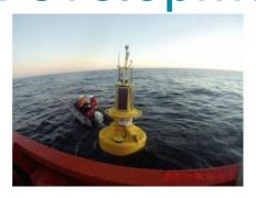
An AXYS WatchKeeper meteorological and oceanographic data buoy has deployed been approximately 60km offshore along the northern coast of Poland in the Baltic Sea. This buoy, procured by Polish developer Baltic Trade and Invest (BTI), will be used as part of the Environmental Impact and Assessment campaign in the Baltic Sea. This campaign will form part of the environmental application for the offshore wind farm development 'FEW Baltic II'.
