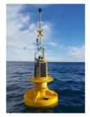
AXYS Technologies Inc (AXYS) is participating in French EolMed wind development initiatives in the zone between Port-La Nouvelle and Gruissan. An AXYS WatchKeeper buoy will be deployed by French company Créocéan on the behalf of QUADRAN, at the location over the next year to gather comprehensive metocean data. This marks the first stage of floating offshore wind development in that area and will gather essential preliminary environmental data to support future design and financing decisions.
