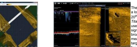
The single beam echosounder has come a long way. First developed in the early 20<sup>th</sup> century in response to the RMS *Titanic* disaster of 1912, early models used a Fessenden oscillator to generate a signal of around 1kHz. The resulting broad beam was suitable for depth measurements and the location of large targets – a huge technological step forward – but incapable of the fine
