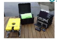
Outland Technology, USA, has presented its Outland 2000 ROV. Boasting twice the power and a heavier payload than the Outland 1000, this model complements the product line. The Outland 2000 comes with a larger frame that allows for more room to add various tools and sonar.
