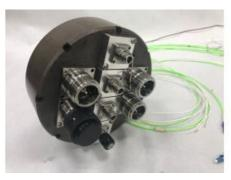
BIRNS, known for developing and manufacturing a range of advanced marine products, has launched a precision testing capability for deep submergence connectors and cable assemblies - an extreme low temperature and extreme depth testing system. The test system successfully allows 48 hour+ continuous testing of connectors and cable assemblies at 6km in a controlled 2°C (±1°C) environment.
