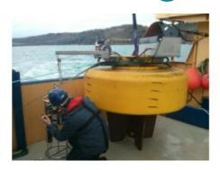
Plymouth Marine Laboratory (PML, UK) has developed a near-surface ocean profiling buoy which scientists can use to gain accurate measurements from the top few metres of the ocean. By suspending instruments below a floating buoy which rises and falls with the swell, measurements can be taken at a constant depth. PML's near surface ocean profiler acts as an instrumentation platform that can be lowered into the sea and left to drift, away from the influence of the â€mother ship'.
