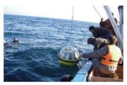
AXYS Technologies (AXYS) has delivered two TRIAXYS Next Wave Directional Wave Buoys to Instituto Nacional de Hidráulica (INH) in Santiago, Chile. This institution is to measure offshore wave characteristics for the purpose of assessing wave energy potential at various sites along the coast of Chile using different calibrated numerical models capable of propagating offshore wave characteristics to near-shore.
