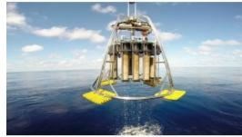
UK-based bespoke marine engineering company Ocean Scientific International Ltd (OSIL) have released a camera system designed to be mounted to deep sea sediment corers. The self-contained system will allow users to record the corer deployment and review the footage on recovery of the corer to check the system has deployed correctly, aid analysis of the sample and re-deployment of the corer, and offer a laser ranged view of the sediment itself via a graticule scale.
